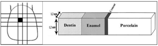
Figure 1. Specimen preparation for microtensile testing
