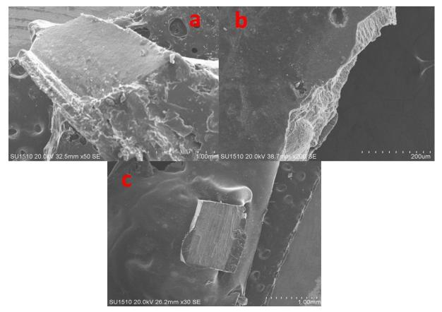
Figure 2. Scanning electron microscope images of the fracture types (a) adhesive failures (AEB), (b) cohesive failure in the bonding resin (CB), (c) cohesive failure in the tooth structure (CT)
